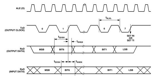
Figure 54. UART Timing in Shift Register Mode
